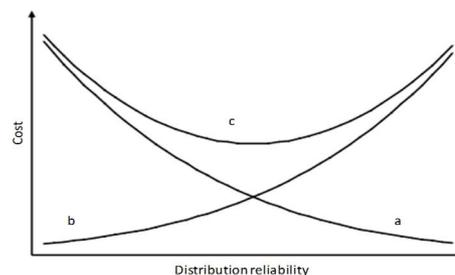
Fig 1. Distribution reliability and cost functions in principle. Adapted from [3].
