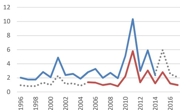
Fig 4. Average interruption duration (blue) and energy-weighted interruption duration (red) [h/customer, year]. Interpolated dot line marked.
