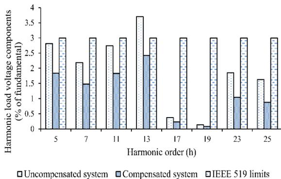
Fig. 4 Harmonic content of the PCC voltage before and after compensation.
