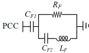
Fig. 1 The equivalent circuit of the C-type filter
