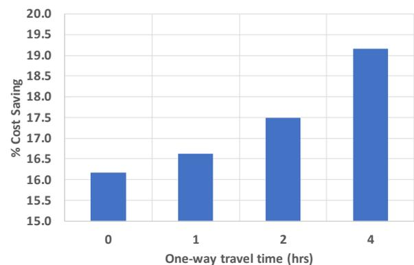
Figure 6: Life cycle cost saving of the chromatography based analyser compared to the infra-red instrument as a function of engineer travel time to carry out repairs.
