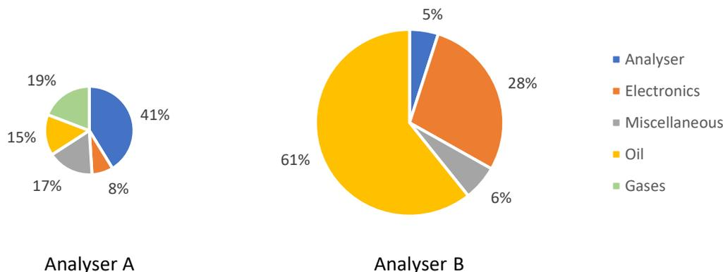
Figure 2: Pie charts showing repair cost breakdown (excluding communications). Pie chart area has been scaled to the average annual repair expenditure on the two different instruments.
