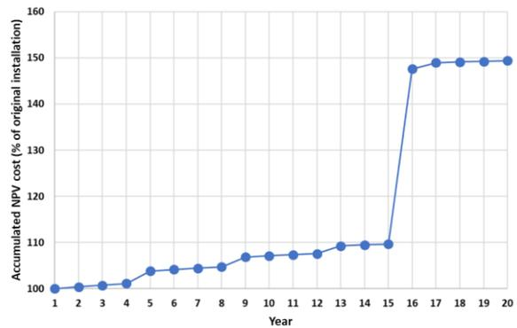
Figure 5: Accumulation of costs through time for Analyser A normalised to the initial installation cost, highlighting periodic analyser replacement.
