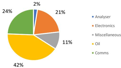
Figure 1: Relative distribution of the type of repairs required on Analyser B population.
