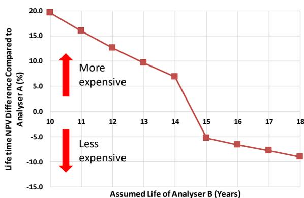
Figure 7: Sensitivity analysis of the effect of Analyser B life on which analyser represents the lowest LLC.
