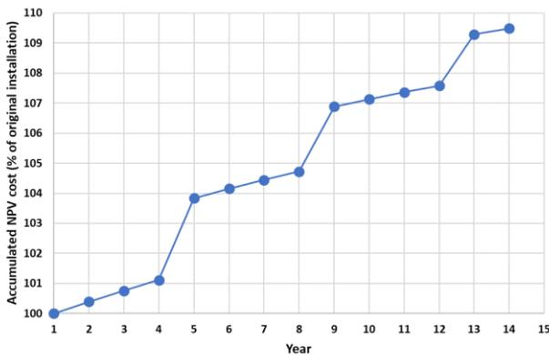
Figure 4: Accumulation of costs through time for Analyser A normalised to the initial installation cost, highlighting repairs and consumable costs.
