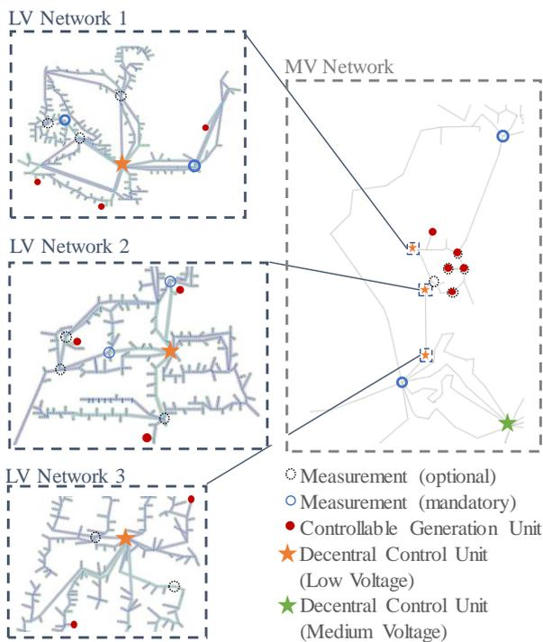
Figure 2 Setup for Field Test and Analytical Assessment
