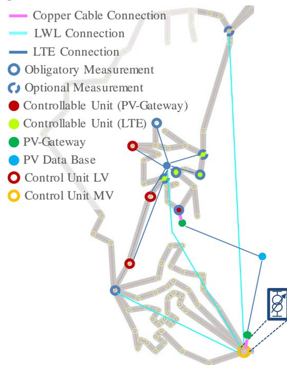
Figure 7 Field Test Setup for Medium Voltage Network
