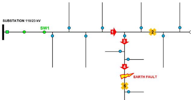
Figure 3: Example of a fault locating procedure
