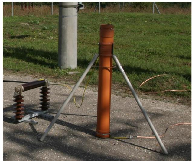
Figure 7: Water resistor of own construction
