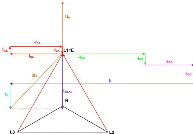
Figure 6: Current measured by the device at a location *between* the substation and the fault + resistor
