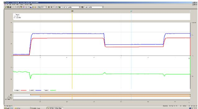
Figure 9: Fault record – fault *before* device's measurement place
