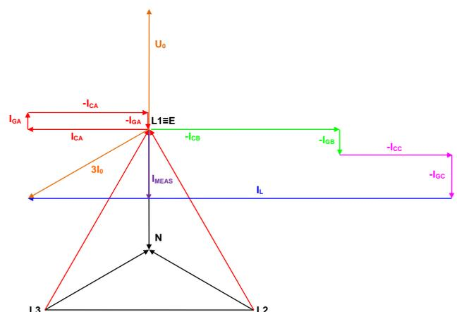
Figure 5: Current measured by the device at a location *between* the substation and the fault
