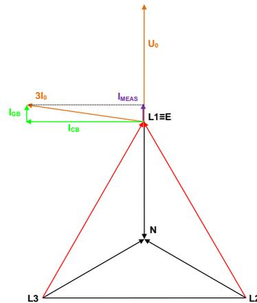
Figure 4: Current measured by the device at a location *not* between the substation and the fault
