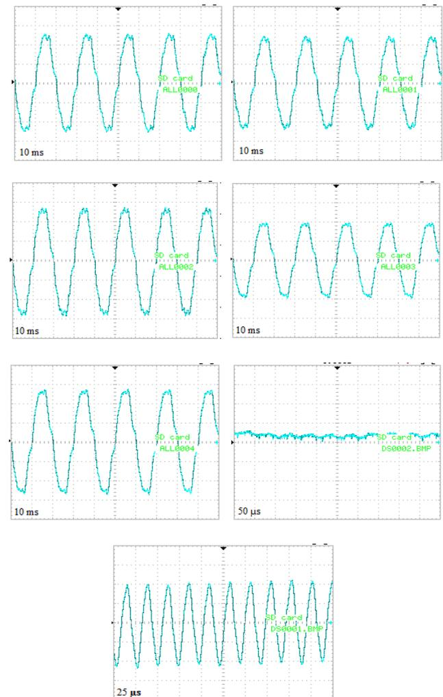
Fig. 4 Light flicker waveform of tested types (from type 1 to type 7 respectively) measured by light flicker portable device and recorded by oscilloscope
