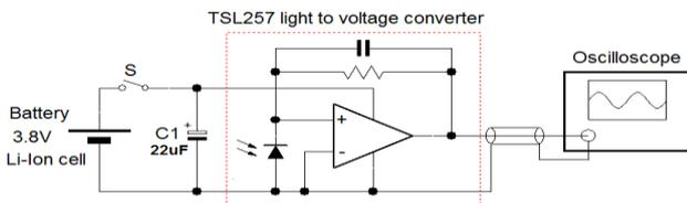
Fig. 1 Light portable measurement device
