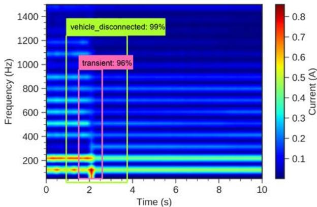
Figure 4: Spectrogram of a transient injected by the disconnection of a BEV
