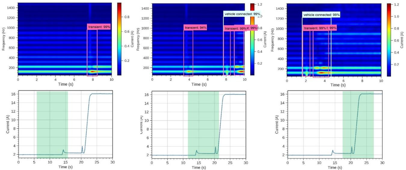
Figure 2: Spectrograms recorded during charging of a BEV (top) processed by the ODA. Current (r.m.s.) during the charging process with the green areas referring to the section of the above spectrogram (bottom).
