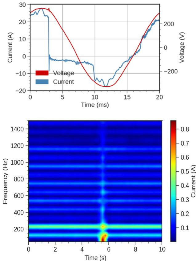
Figure 1: Transient in waveform data (top). Transient in the spectrogram of aggregated harmonic r.m.s. values (bottom)
