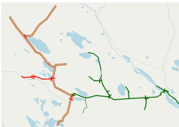
Figure 5: A fault has occurred. The solid red line indicates a line without power. The red line surrounded by green indicates a line where power can be restored by isolating the fault. The red dot is the fault position.
