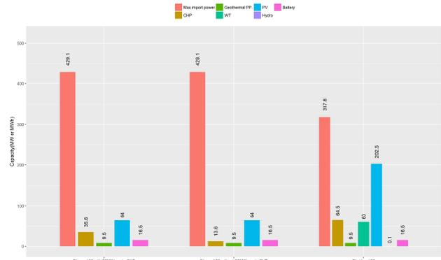
Depending on the presence of the waste incineration CHP, the capacity of each case is much differ. For Case 3, in order to avoid using external input, which is relatively expensive, many renewable resources are installed.
