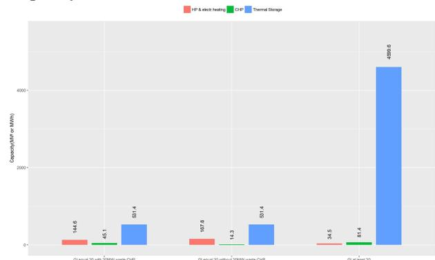
For case 1, CHP covers much of a heat demand, the capacity of other resources is relatively small. However, the case 3 has a considerably high capacity of the heat storage, because the installation cost of the heat storage is cheap, and it is economical to store the heat from CHP in a large amount to assist heat supply in winter.
