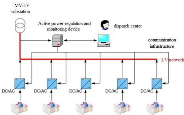
Fig. 2 Centralized system for active power regulation
