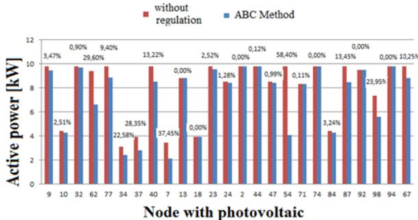
Fig 7. Comparison of total and curtailed active power of each photovoltaic
