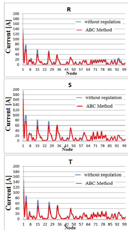
Fig. 6 Comparison of currents in all branches before and after application of the proposed method
