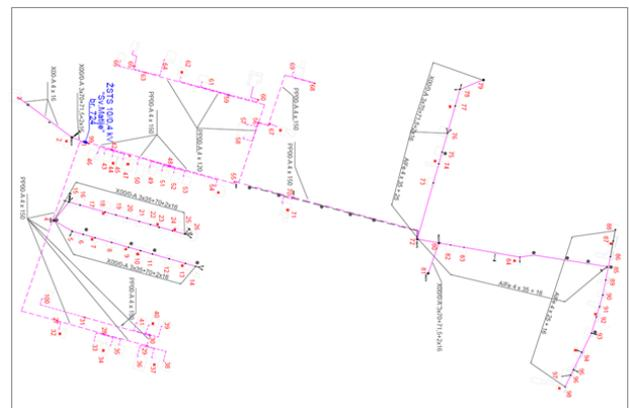
Fig. 3 Real LV network from substation 10/0,4 kV sv. Matije, Sibirj near Slavonski Brod, Croatia [8]
