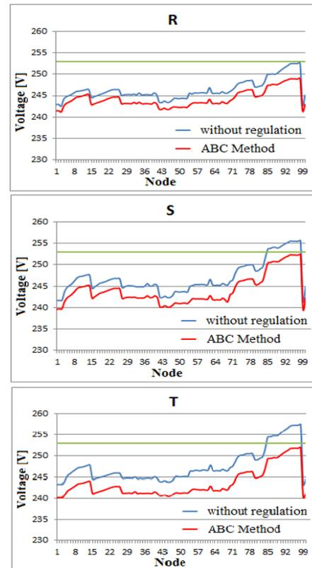
Fig. 5 Comparison of voltage profiles before and after application of the proposed method
