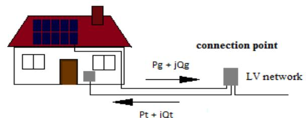
Fig. 1 Simplified model of a prosumer with roof photovoltaic
