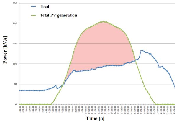
Fig. 4 Comparison of daily loading curve and total photovoltaic generation curve for the observed LV network [8]
