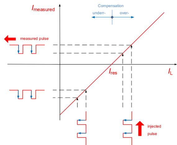
Fig. 7 Reduced amplification of the pulse near to the resonant-point due to wattmetric current
