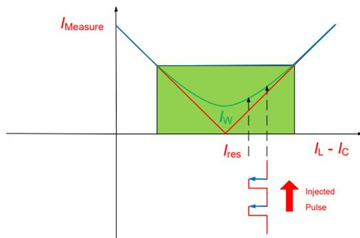
Fig. 6 Hiding of the pulse due to harmonics in the zero-sequence current
