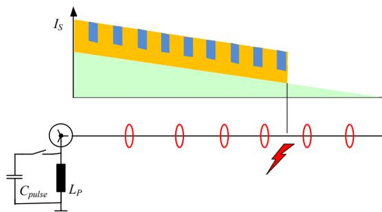
Fig. 2 Principle of the standard pulse method, over-compensated grid
