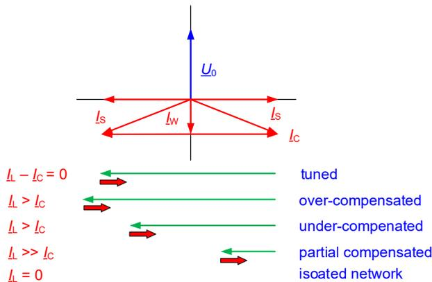
Fig. 8 Direction of the capacitive pulse not depending on the different types of compensation
