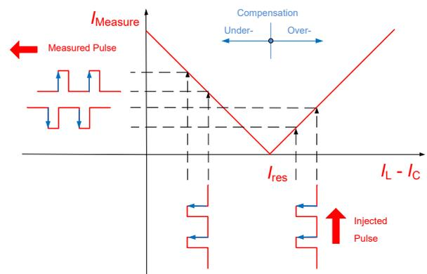
Fig. 3 Asymmetric pulses for the case of high ohmic earth faults at the fault location as function of the compensation
