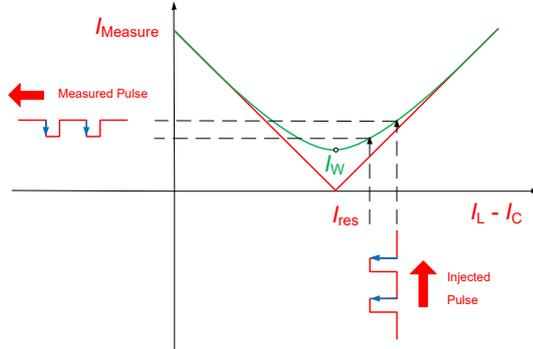
Fig. 5 Reduced amplification of the pulse near to the resonant-point due to wattmetric current
