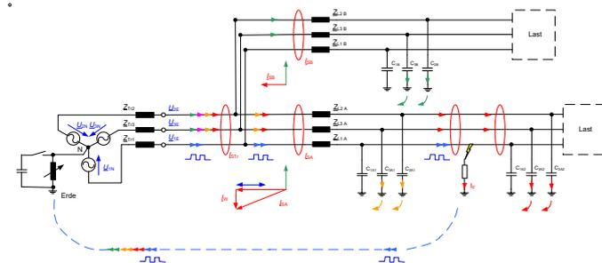
Fig. 1 Compensated network with the standard pulse method
