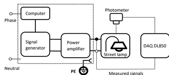
Fig.1 LED street lamp testing mock-up
