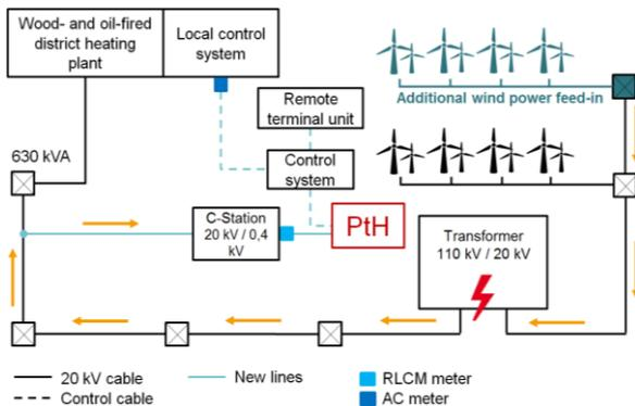
Figure 1: Technical integration scheme of the PtH asset
