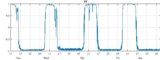
Fig. 14. Power factor measured on PCC.
