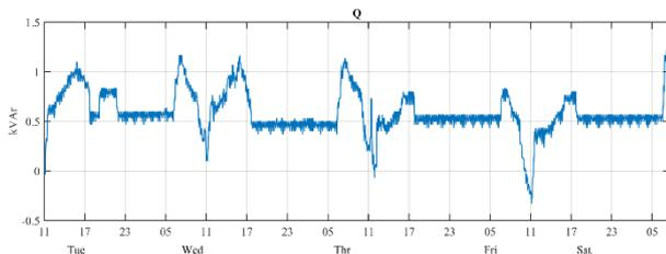
Fig. 13. Reactive power measured at PCC.
