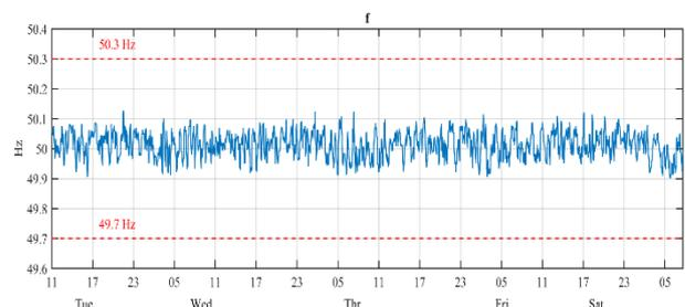
Fig. 5. Voltage Frequency variation graph.
