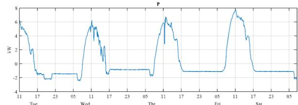
Fig. 12. Active power measured at PCC.
