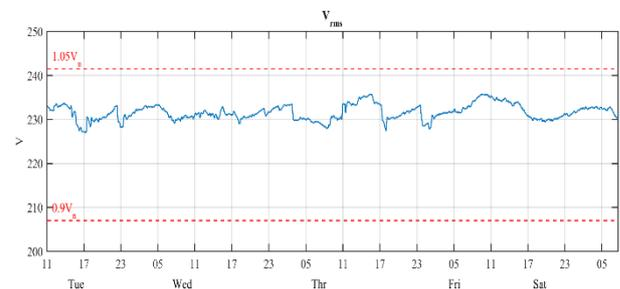
Fig. 4. RMS voltage at PCC
