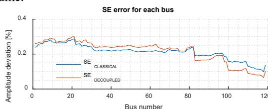
Fig 10: SE voltage error comparison, same time step and phase
