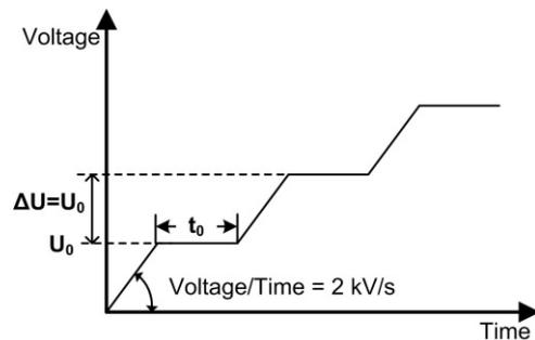
Fig. 10 Step-up voltage method
