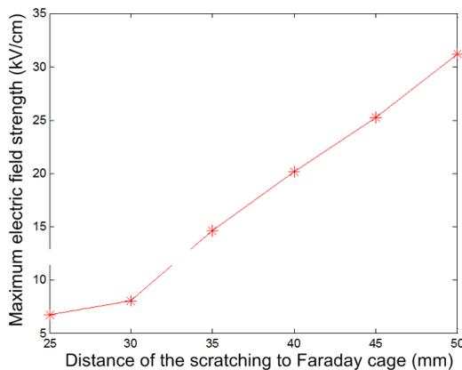
(b) Relation between the maximum electric field strength and the position of scratching defects
