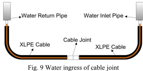
Fig. 9 Water ingress of cable joint
