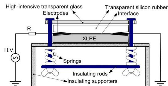
Fig. 5 Schematic of surface breakdown test at the interface of XLPE and SiR
