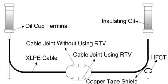
(b) Schematic of PD test
