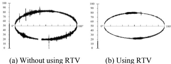
Fig. 7 PD signals of cable joints based on pulse current method with and without using RTV adhesive
