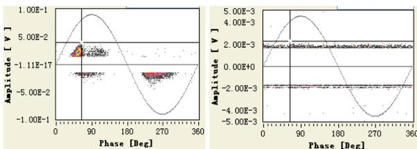
Fig. 8 PD signals of cable joints based on electromagnetic coupling method of high-frequency current with and without using RTV adhesive
