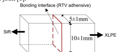
Fig. 2 Schematic of mechanical test
