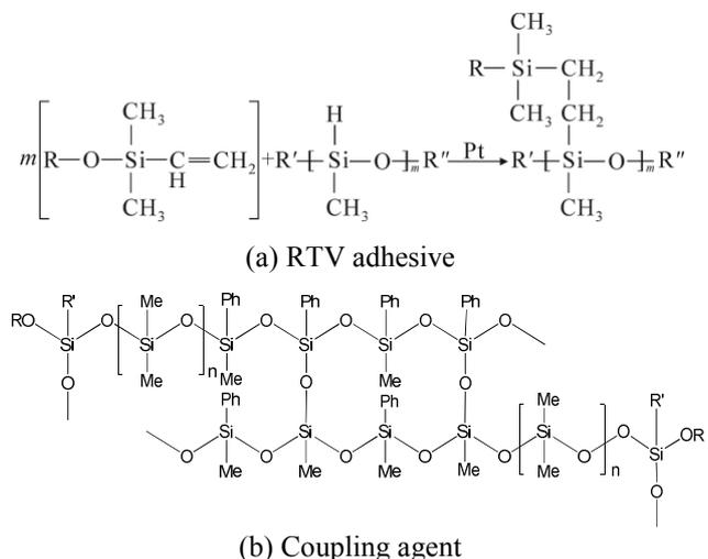
Fig. 1 Molecular structure of RTV adhesive and its coupling agent
