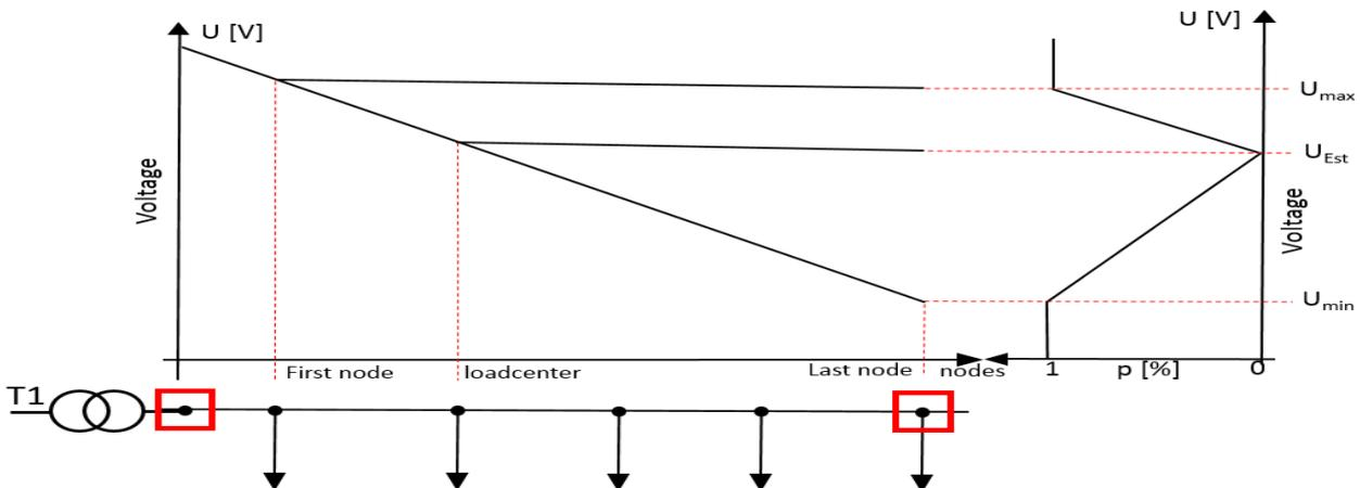
**Figure 4:** Calculated voltage limits and probability diagram
