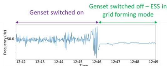
**Figure 4** - Stability of frequency in operation
