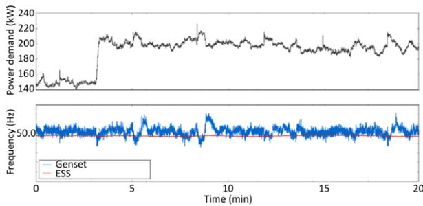
**Figure 3** - Comparison of the quality of frequency generated by the gensets and the ESS
