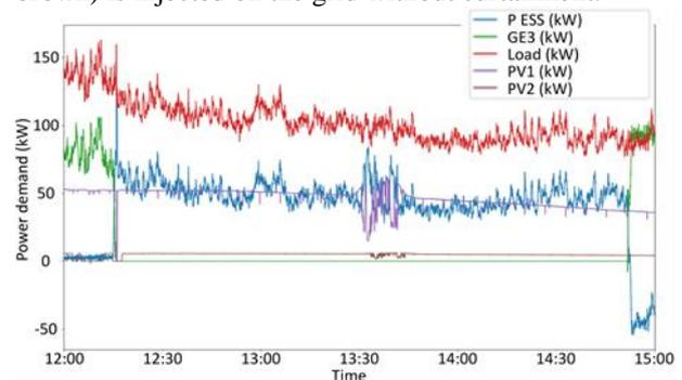
**Figure 5** - Islanding mode of the ESS
