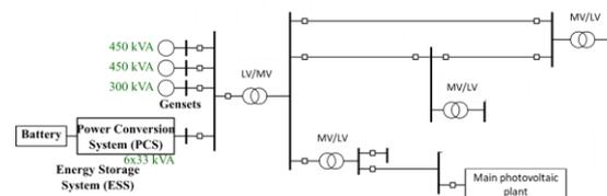
Figure 2 - Single Line Diagram of the island's grid
