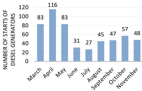
**Figure 6** - Number of starts of diesel generators for each month (2017)
