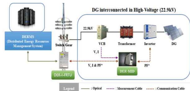
Fig. 6. The configuration of High-Voltage system
