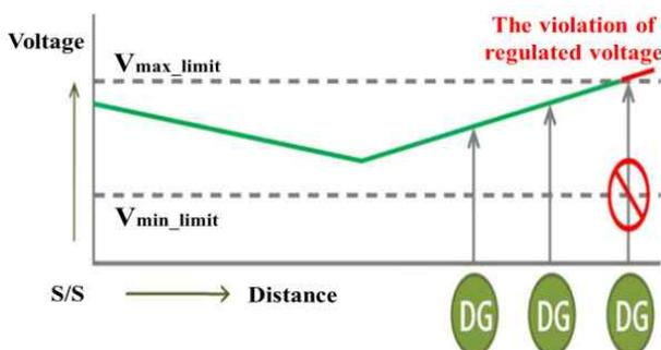
Fig. 1. The D/L voltage profile from S/S
