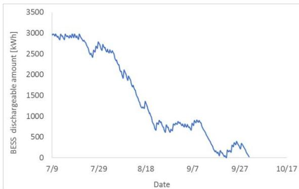
Fig. 7. Trend of BESS capacity (SOC) in the event of insufficient power generation
