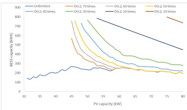
Fig. 9. Relation between PV output and BESS capacity
