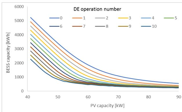
Fig. 8. Relation between PV capacity, number of DE operations and required BESS capacity
