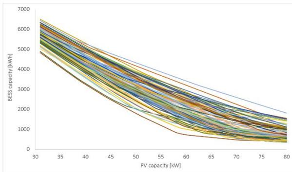
Fig. 6. Combination of operable PV and BESS capacity
