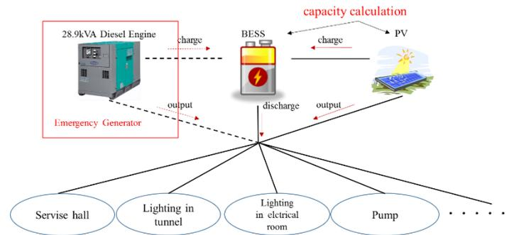
Fig. 1. Outline of the off-grid power supply system
