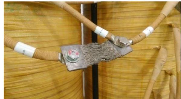
Fig. 6. Turn-to-turn short circuit
