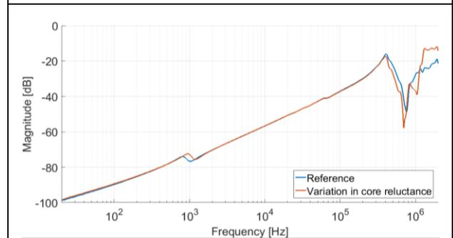
**Fig. 14. Capacitive inter-winding (H1-X1).**
