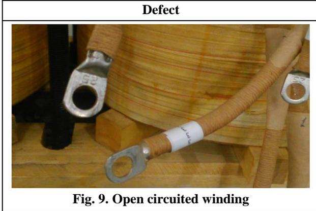
**Fig. 9. Open circuited winding**
