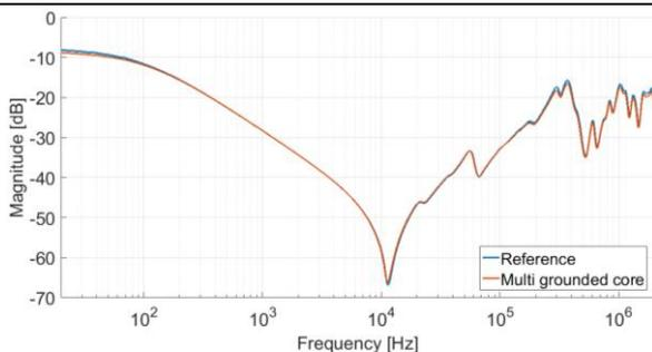
**Fig. 17. End-to-end short-circuit (H3-H2).
