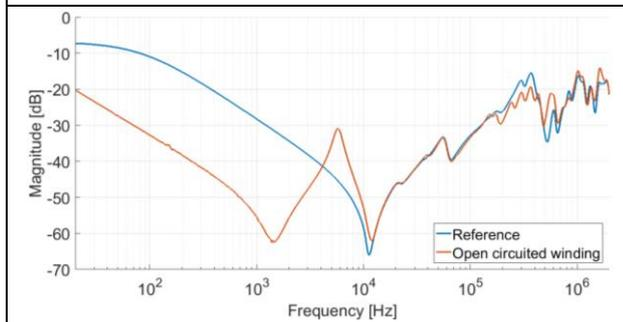
**Fig. 10. End-to-end short-circuit (H3-H2).
