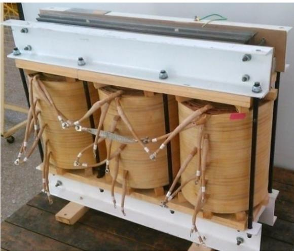
Fig. 5. Transformer used to emulate mechanical defects
