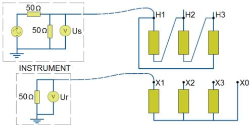
Fig. 3. "Capacitive inter-winding" test type
