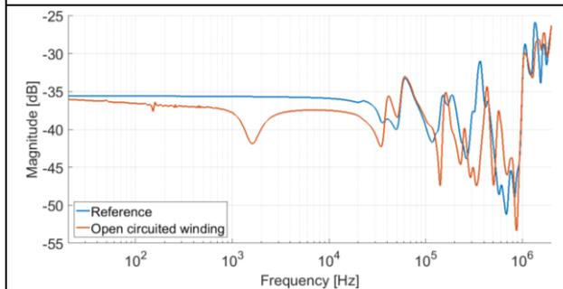
**Fig. 11. Inductive inter-winding (H2-X2).
