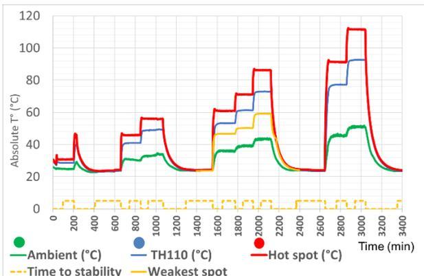
**Figure 8:** Thermal measurements of insulated parts
