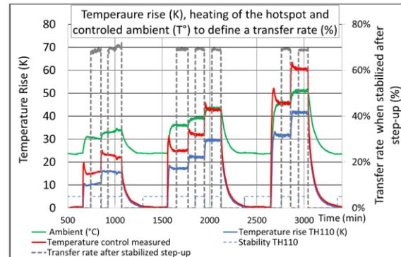
**Figure 9:** Transfer rate after stabilized step-up
