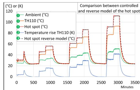
**Figure 10:** Calculated hot spot of a connection
