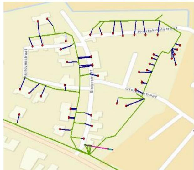
**Figure 1:** A map of De Veldegge. The electricity cables are shown in green, the connection cables in blue, the houses in red, and the transformer is in pink.
