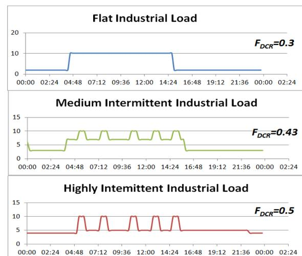
Figure 1. Industrial load profiles with different  $F_{DCR}$
