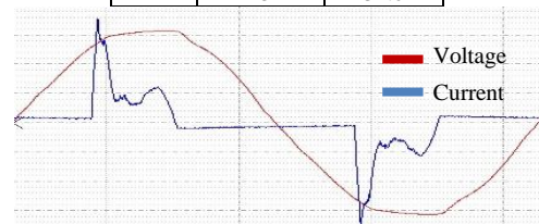
Figure 1. Voltage and current waveforms for lamp type 1-A.
