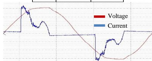
Figure 8. Voltage and current waveforms for lamp type 6.
