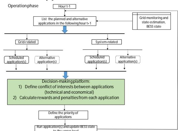
Figure 2. An operating phase of a BESS scheduling for multiple tasks (an intra-day market and grid tasks in addition to a day-ahead market) [6]
