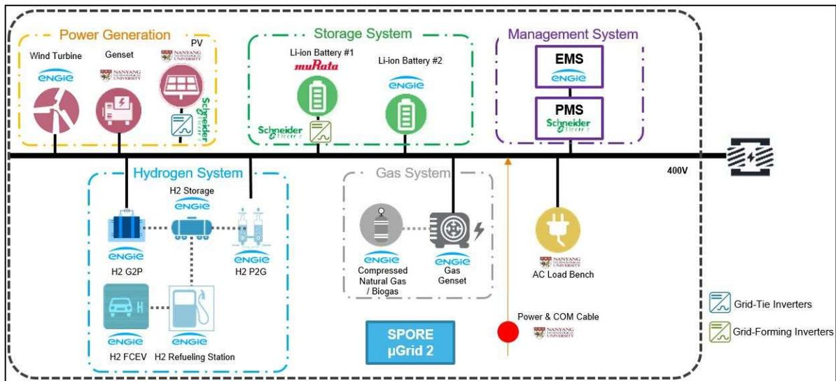
Figure 2 : Schematic of the SPORE microgrid
