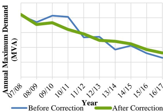
Fig. 3: Corrected demand trend at example substation
