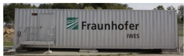
Figure 2. Mobile test equipment (LVRT test container)
