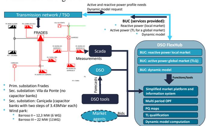
Figure 1: Flexibility Hub simplified architecture
